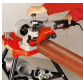
Use with roll grooving tool ROGROOVER
