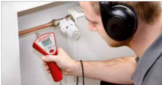
Acoustic leak detection of heating installations
