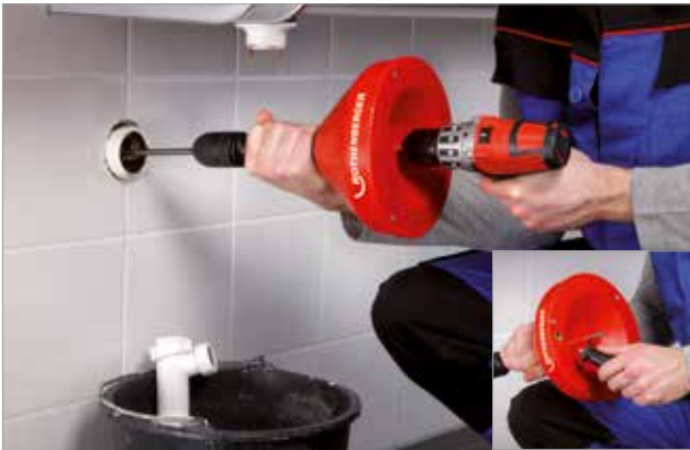
Electrical operation with cordless drill
