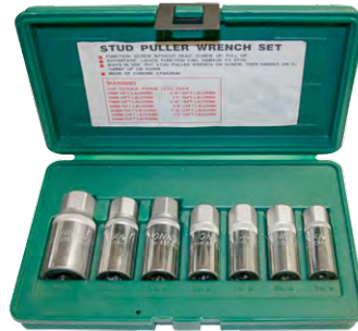
JOA432 AG010061 7Pc Stud Puller Wrench Set Excellent to use with screws without heads. Quick operation without any damage to the stud. Just put the stud puller wrench on a screw, then add the handle and turn in desired direction. Size: 5, 6, 7, 8, 10, 12, 14mm Warning: Use torque range no more than: 5mm - 15Ft/Lbs (20NM) 10mm - 15Ft/Lbs (33NM) 6mm - 15Ft/Lbs (20NM) 12mm - 15Ft/Lbs (33NM) 8mm - 15Ft/Lbs (20NM) 14mm - 15Ft/Lbs (33NM)
