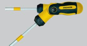
Locking of the handle in normal and angled position at the push of a button. Reverse lever for clockwise and anticlockwise rotation by turn-ing the shift ring. In centre position the ratchet function is eliminated. Autolock system: Bits are form-locked automatically when inserted by means of a spring and a magnet. To release, slide ejector backwards.
