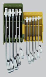
With ratchet mechanism and reverse lever on the ring end for clockwise and anticlockwise rotation. No swapping over: a real time saver. Ideally suited for working on flat surfaces due to its 15° offset ring side. Practical foldable holder offering a clearly marked place for storage of each spanner. The ideal companion for construction site work. Holder also provides holes for wall-mounting in the workshop. With clearly readable sizes. Organised forever!
